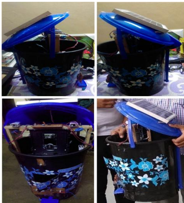
Fig. 7 Prototype of the solar-powered waste compactor
